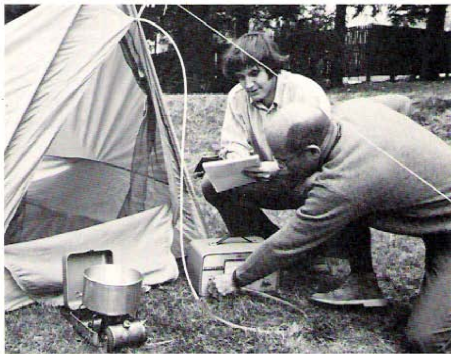
Authors Joseph Kohler (left) and Robert Wagner set up an analyzer inside a tent to measure carbon monoxide dangers of backpacking stoves. The tent was made of breathable nylon, pitched without rain fly to simulate actual mountaineering use. During the tests, the tent's rear vent was open and the tent entrance was zipped partially open. After five minutes most stoves had filled the tent with dangerous quantities of carbon monoxide.
